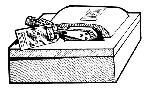
Electrical Device That Is Properly Labeled, Tagged and Locked out
