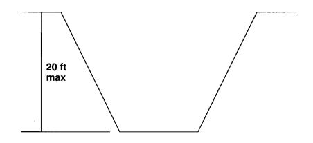
**Benching:** Benching relies on the maximum allowable slope principal but employs one or more vertical sided portions. Benching must be designed by a "competent person" taking soil type, trench depth, and other conditions into account. Appendix B of OSHA 1926 Subpart P displays some suitable benching configurations. Benching is for Type A and cohesive Type B soils. Benching for Type A soil is illustrated below.
