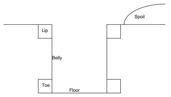
The **lip** usually refers to the area at the top of both sides of the trench, and the **toe** the area on both sides of the floor of the trench. The **belly** refers to the space between the lip and toe of the trench, and the **spoil** refers to the soil, rocks or other materials removed from the trench. The spoil pile must be at least 0.61 m away from the lip of the trench.
